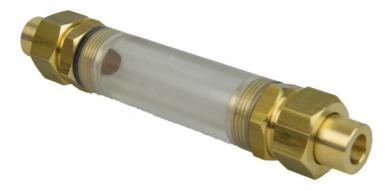
The **pipeline isolator** is used to electrically isolate / separate pipelines in individual departments or areas, such as operating theaters or intensive care units in hospitals and clinics, from other pipelines within the central medical gas supply.
