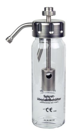
The function of the septic fluid jar overflow protection is to protect as second stage the ejector or the vacuum regulator against contamination. If the maximum filling capacity of 200 ml is exceeded, a float is closing the supply to the vacuum source.
